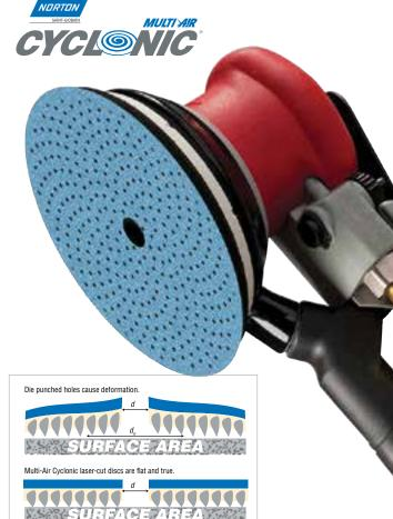
Improved Dust Extraction / Increased Productivity The upgrade to precise, flat, laser-cut holes instead of die-punched holes, dramatically increases surface area contact allowing Norton Multi-Air Cyclonic discs to improve productivity by 32% versus conventional multi-hole sanding and by 60% versus non-vacuum sanding.
