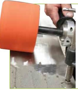
Portable belts are ideal for all your metal and woodworking applications. Choose 36 -50 grits for rough/heavy-duty applications, 60 - 100 for intermediate, and 100 - 220 for finishing/polishing applications.
