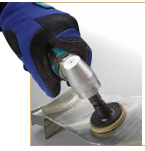
Made from non-woven synthetic fiber mesh, which is impregnated with abrasives and bound with resins, non-woven wheels are designed to create desired surface finish where little or no stock removal is required. The industry's broadest offering is available for light stock removal, deburring, blending, finishing and polishing. Non-woven wheels have an open mesh construction that is waterproof, washable, conformable and non-loading.
