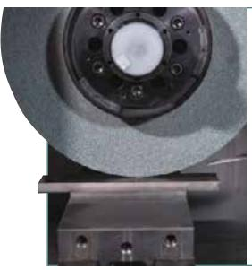
These sharp silicon carbide, vitrified wheels are used for grinding non-ferrous applications.
