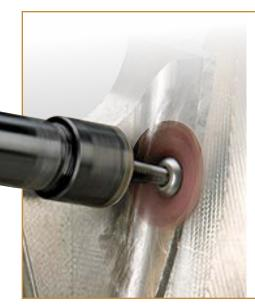
Square pads, cross pads and overlap slotted discs are all used on high-speed pneumatic tools for deburring, blending, cleaning, and polishing applications. All of these abrasive specialties are designed for applications in small, tight, hard-to-access locations on parts that are being finished.
