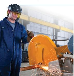
The Norton stationary saw reinforced cut-off wheel line consists of Type 01/41 straight 10" - 24" wheels, designed to fit on fixed-base stationary saws that are free-standing or mounted on a workbench.
