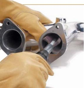
Flaps of abrasive cloth are stacked, inserted into a holder, and then attached to a mandrel. The flaps are designed to break down during use and reveal the next layer of abrasive.
