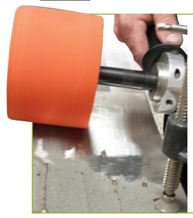
Portable belts are ideal for all your metal and woodworking applications. Choose 36-50 grits for rough/heavy-duty applications, 60-100 for intermediate, and 100-220 for finishing/polishing applications.
