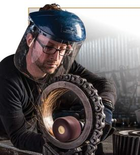
Non-woven surface finishing flap wheels are an ideal choice for a wide variety of blending and finishing applications common in the metal fabrication, welding and polishing industries. Flap wheels are conformable to intricate shapes and contours. Designed to deliver a consistent finish with a uniform rate of cut, flap wheels wear away continually exposing fresh abrasives.
